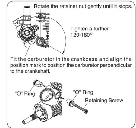
1. Loosen the retainer screw, rotate the carburetor to its correct position and make sure that it is pressed well down into the intake boss, compressing the rubber gasket, before retightening screw.
