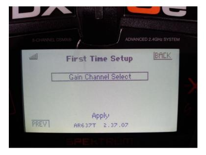
Scroll curser box over 'Gain Channel' and press, then scroll to 'AUX3', press to lock in. Scroll down to 'Input' and press, then scroll to 'RKnb', press to lock in. Scroll curser box over 'Next' and press the roller.
