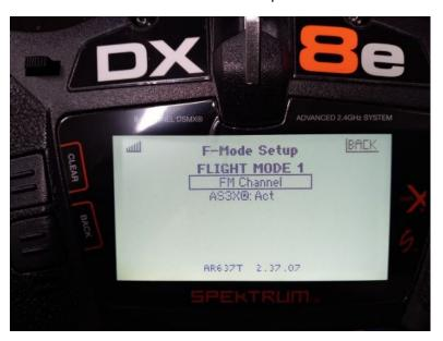
Scroll curser box over 'FM Channel' and press, then scroll to 'AUX2', press to lock in. Scroll down to 'Input' and press, then scroll to 'G', press to lock in. Scroll curser box over 'Next' and press the roller.
