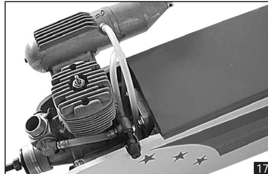
5) Mount the muffler to the engine using the mounting bolts provided with your engine.
