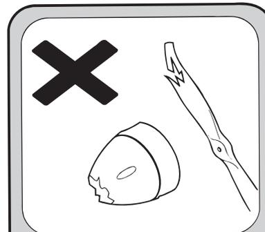
**NEVER** use damaged or deformed propellers or spinners.
