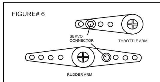
8) Connect the servo to your radio's receiver and turn on the system. Set the trim tabs on the transmitter to neutral and center the servo arms. The elevator and rudder servo arms should be perpendicular to the servos. For the throttle, we suggest setting the throttle trim tab and the throttle stick to the lowest setting which will be used to shut off the engine. Also mount the servo arm about 45° back from perpendicular. **See photo # 7 below.**
